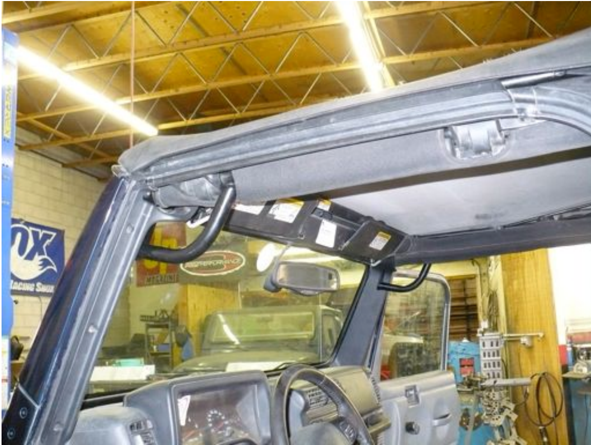
Completed install of PPM-5804 TJ Front Grab Handles
