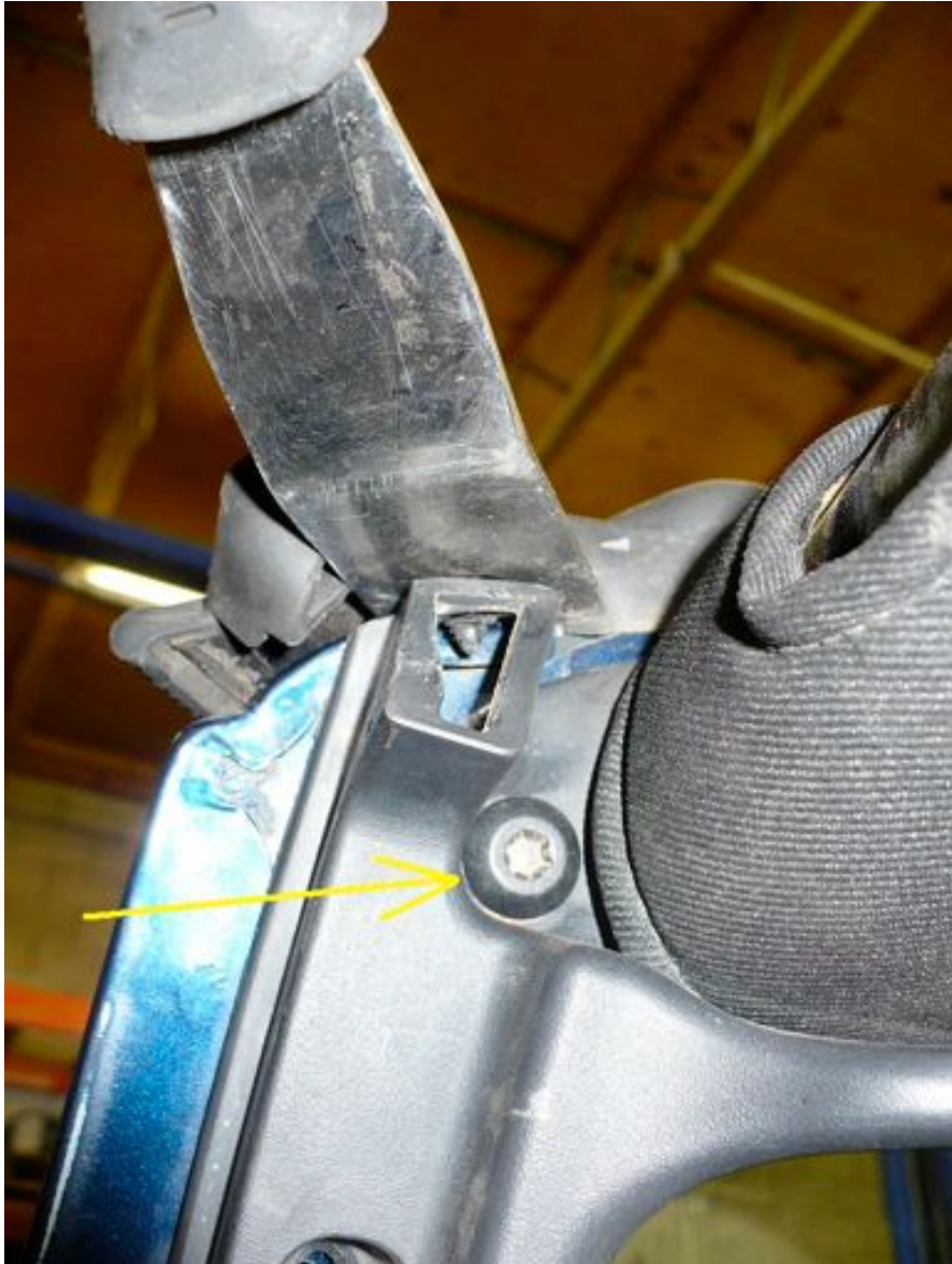
Plastic barb fastener at top of A-pillar trim
